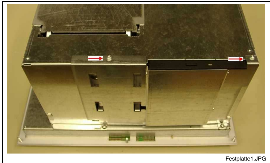
Fig. 8-3: Retaining screws of the hard disk frame
